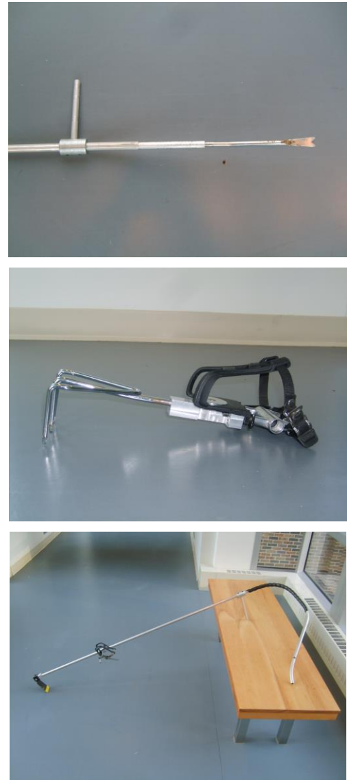
Fig. 7.24. The custom gardening tools. From top to bottom: the working end of the weeding tool, shoe tool for raking, integrated body-rod with hoeing tool.
