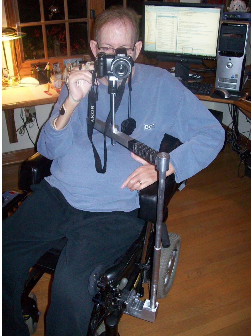
Fig. 7.14. The client using the camera with the Birdie Buddy.
