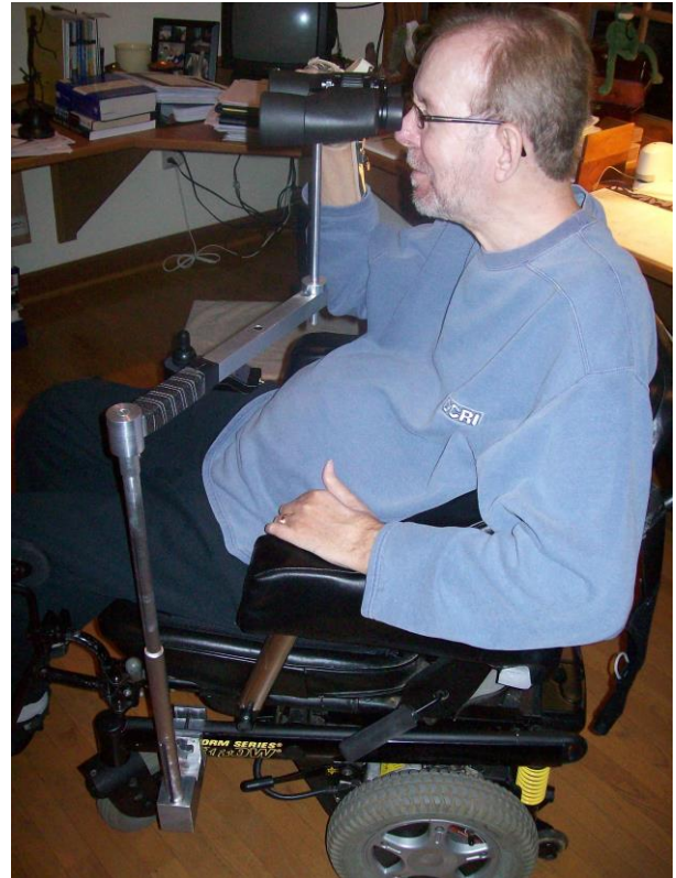
Fig. 7.13. Birdie Buddy with binoculars attached to client’s wheelchair.
